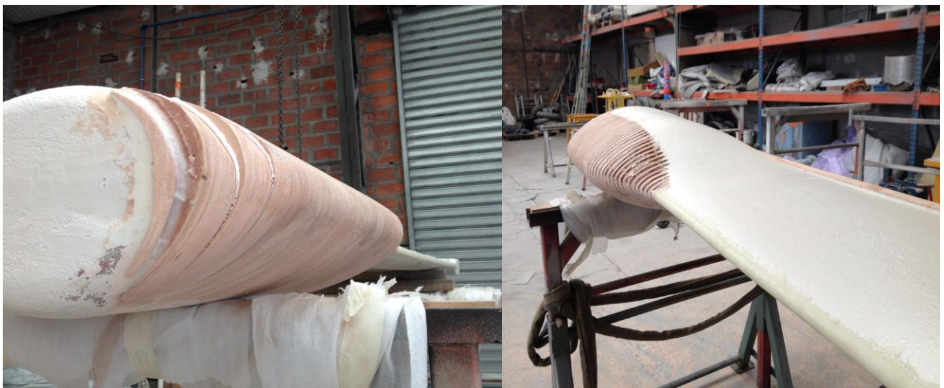
The Paroa 34's backwards-lifting cast-iron keel, with its bumper
